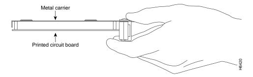
Step 6 Place the port adapter on an antistatic surface with its components facing upward, or in a static shielding bag. If the port adapter will be returned to the factory, immediately place it in a static shielding bag.
